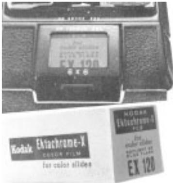
9) The film indicator frame is designed to accept the end flap of the empty film box to indicate the type of film loaded in the film back.
